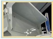
Both the DuraTuff® LD and DuraTuff® MD feature adjustable-height cabshields that accommodate a variety of chassis cab heights and make mounting the bodies easier.
